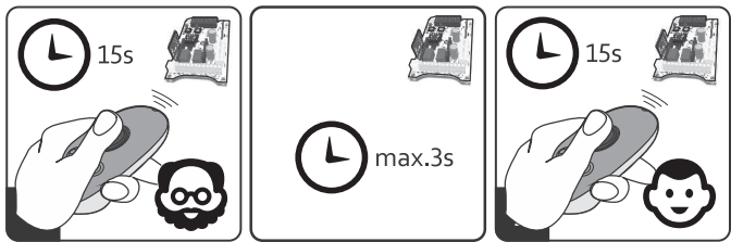
Fig.4 Remote adding the remote control 15s/15s.
